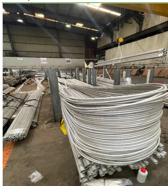
Exhibit 33: U tubes manufactured at the plant
